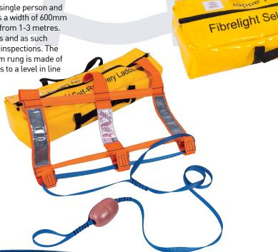
The Fibrelight Self Recovery Ladders are constructed using GRP rods enclosed in flanged tubular webbing which together create an incredibly strong structure. The ladders exceed the ISO 799 strength test which is part of the SOLAS approval programme. The Fibrelight Self Recovery Ladder has been successfully tested for thermal ageing, weathering, UV light and oil resistance.
